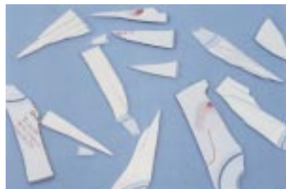
Figure 1 Educational compact disc burst into sharp-edged splinters after extreme bending by a 9 year old child. Warnings should be attached to CD cases.
